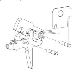
\*Installation of pin keeper shown
