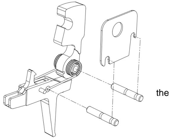
*\*Installation of pin keeper shown*
